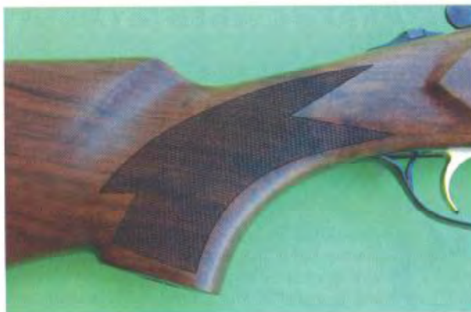
The checkering, likely created via a sophisticated laser machine, is well done.
